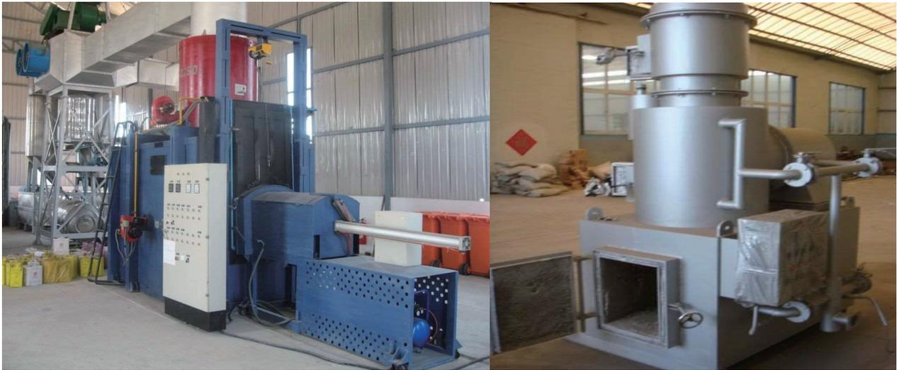
Figure 16 Incinerator Model FSI-150 (left); Incinerator Model LDF-500 (LDF-100) (right)
